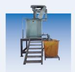
The tank mixer contains an impeller that combines raw materials such as clay, kaolin, feldspar and quartz to prevent sedimentation
