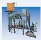
The machine uses electricity to create a magnetic field within the chamber to draw out metal from the liquid in the clay.
